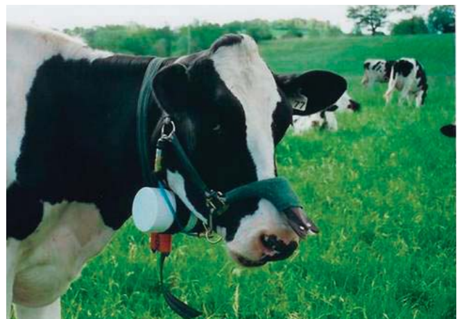
Special halter used to sample cow's breath for methane emissions
